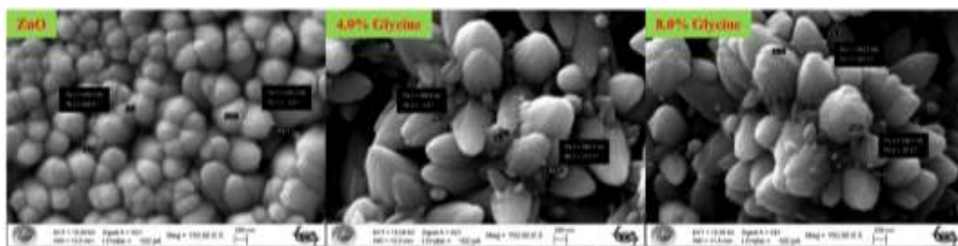
Figure 2. Magnified SEM microimages for the ZnO films synthesized with and without glycine.
